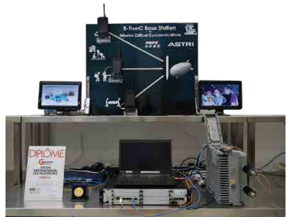
ASTRI leveraged on 5G technology to develop a B-TrunC base-station for mission critical communication.
