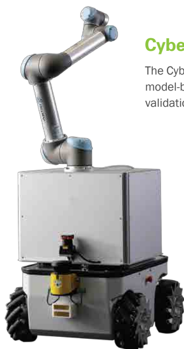
Collaborative Mobile Manipulator is one of ASTRI's advanced robotic systems designed for smart factories in future.
