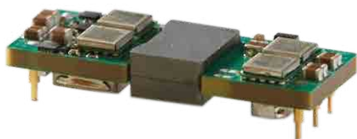
3D packaging is one of the advanced techniques ASTRI employed in R&D of integrated power modules.
