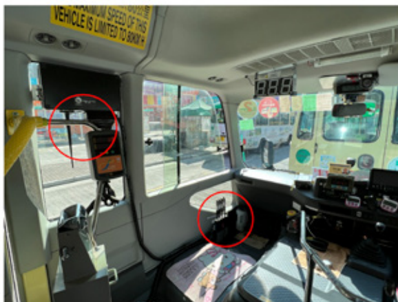
A 5G On-Board Unit (OBU) deployed on a green minibus
