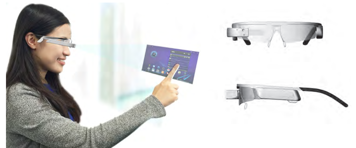
ASTRI's Head-mounted Display (HMD) enables finger touch sensing on air 應科院頭戴式顯示設備實現手指虛擬觸控
