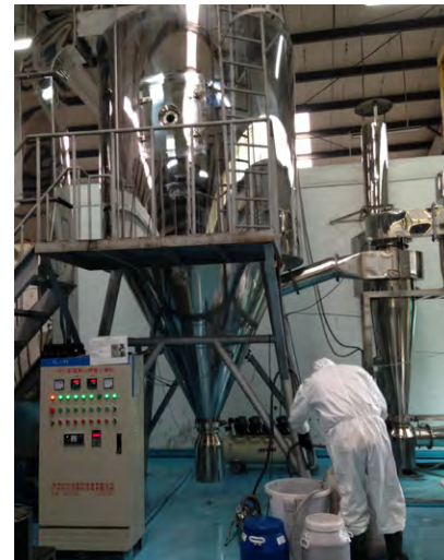
Spray drying treatment of lithium rich cathode materials 富鋰正極材料的噴霧乾燥處理
