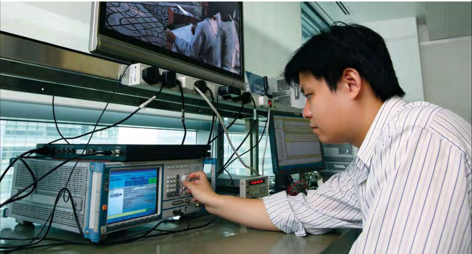
Engineer testing the DTMB receiver system 研發工程師正在實時測試DTMB接收機
