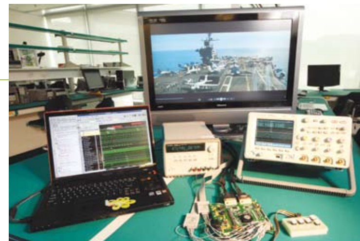
Test setup for LED backlight control ASIC. LED背光源控制晶片之測試組件。
