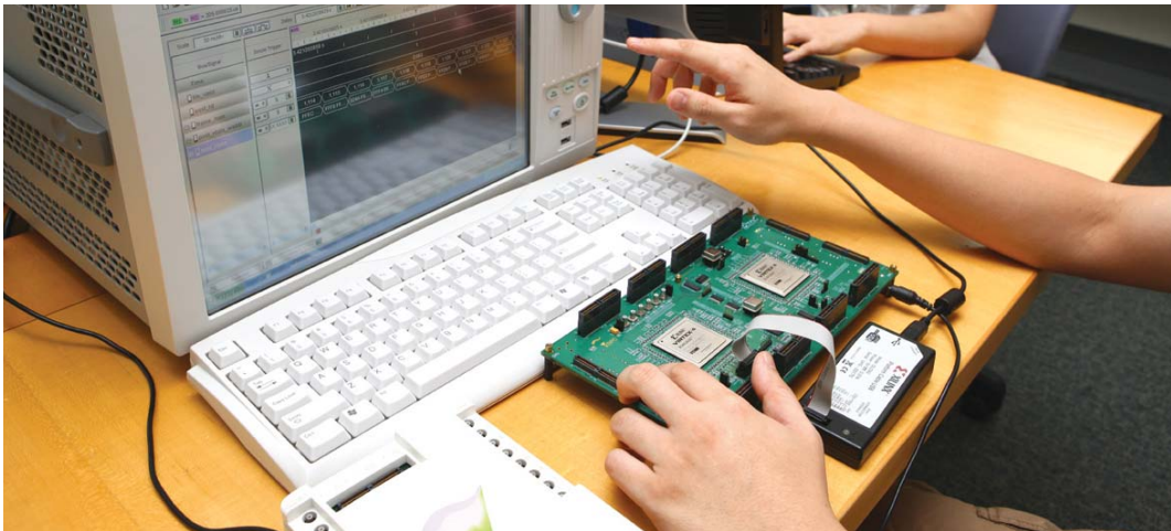
FPGA testing for the development of DTMB Demodulator Chip
